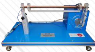
RYC-BB. System kulka na belce (Ball & Beam)
