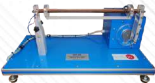
RYC-BB. System kulka na belce (Ball & Beam)
