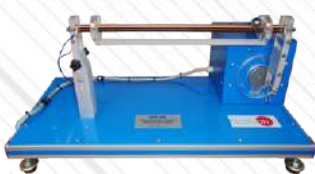
RYC-BB. System kulka na belce (Ball & Beam)
