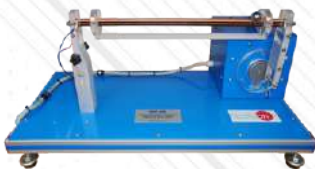
RYC-BB. System kulka na belce (Ball & Beam)
