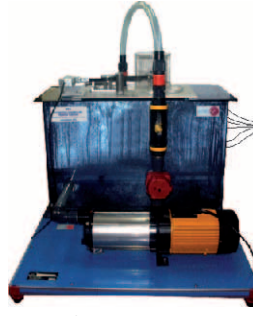
① Unit: TFC. Francis Turbine
