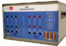
TPPT. Three-phase Power Transformer Unit
