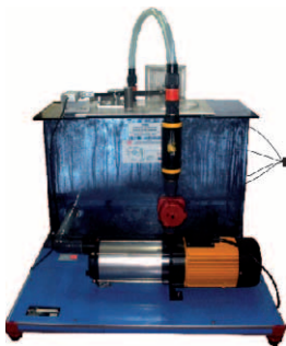
① Unit: TFRC. Radial Flow Turbine
