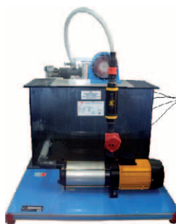
① Unit: TPC. Pelton Turbine
