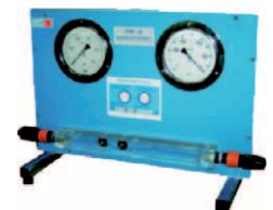
FME19. Cavitation Phenomenon Demonstration
