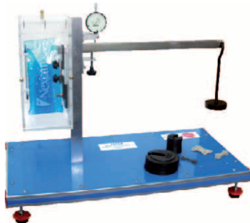
EEDB. Brinell Hardness Testing Unit
