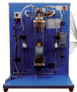
① Unit: TCGC. Film and Dropwise Condensation Unit
