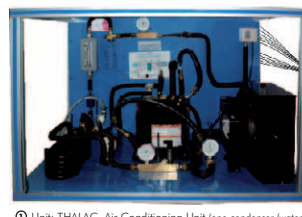
① Unit: THALAC. Air Conditioning Unit (one condenser (water) and one evaporator (air))
