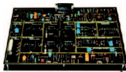
EDICOM 6. Optical Fibre Transmission and Reception
