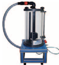
FME04. Orifice Discharge
