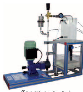
① Unit: PBRC. Piston Pump Bench
