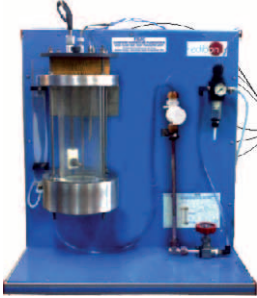
① Unit: TLFC. Fluidisation and Fluid Bed Heat Transfer Unit
