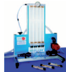
FME24. Unit for the study of Porous Beds in Venturi Tubes (Darcy's Equation)
