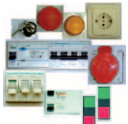
KI9. Kit of People Safety Against Indirect Electrical Contacts in TT Neutral Regimen
