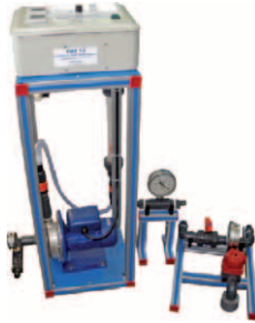
FME13. Centrifugal Pumps Characteristics
