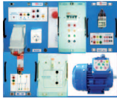
AI7. Automatic Change of Speed of a Dahlander Motor with Change of Direction
