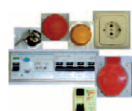
KE4. Kit of Test Unit for Differential Automatic Switches
