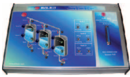
PLCE-PLT. Filling Process of Tanks
