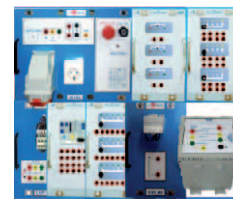
AE7. Multi-Functional Electrical Protection Station
