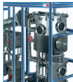
① Unit: QEDC. Batch Solvent Extraction and Desolventising Unit
