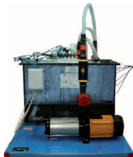
① Unit: TFAC. Axial Flow Turbine
