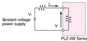
The resistance remains constant despite the change in the voltage and current.
