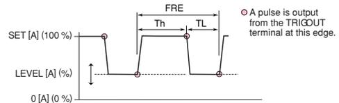
[Setting parameters] ■ Operation mode: CC and CR ■ Duty factor: 5% to 95%, in steps of 0.1% ■ Frequency setting range: 1 Hz to 20 kHz ■ Frequency setting resolution: 0.1 Hz for 1 Hz to 10 Hz; 1 Hz for 10 Hz to 100 Hz; 10 Hz for 100 Hz to 1 kHz; 100 Hz for 1 kHz to 20 kHz ■ Frequency setting accuracy: ±(0.5% of set)
