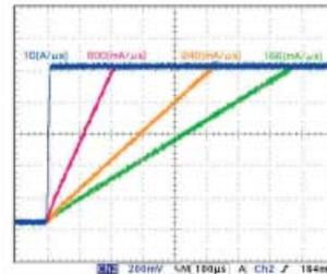
\* Shift in the current waveform with the change in the slew rate
