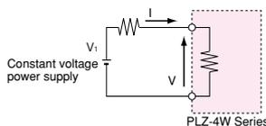
The power (current  $\times$  voltage) remains constant despite the change in the current and voltage.
