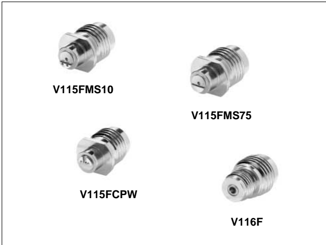
V115FMS75* Integrated V Female solder-in connector, with ground lip, DC to 65 GHz. Compensated for Microstrip. For use with 0.19 mm (7.5 mil) substrates.
