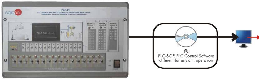
① Unit: PLC-PI. PLC Module for Unit Operations Control (for working with EDIBON Computer Controlled Units)
