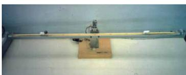
Unit for the study of the stabilization of a naturally unstable system, and control of the position of the ball.
