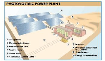
Photovoltaic Power Plant
