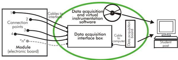
EDAS/VIS is the perfect link between the modules and the PC. With the EDAS/VIS system, information from the modules is sent to the computer. There, it can be analyzed and represented.
