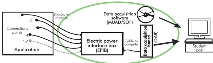
MUAD is the perfect link between the application and the PC. MUAD is a continuous data acquisition system with virtual instrumentation, that measures, analyzes and represents the parameters involved in the process.
