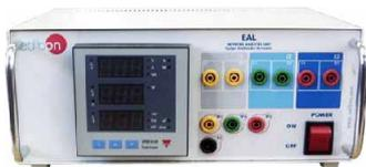
This unit shows the main electric parameters on the electric network through the interface and an easy parameter selection.
