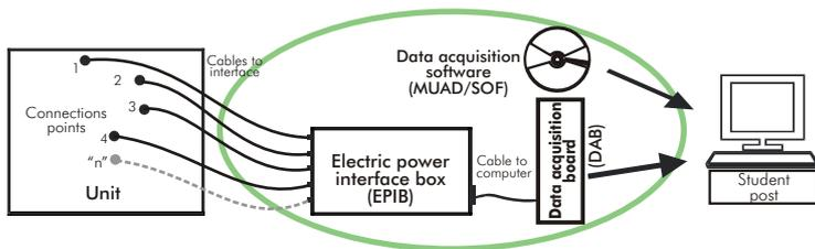
MUAD is the perfect link between the unit and the PC. MUAD is a continuous data acquisition system with virtual instrumentation, that measures, analyzes and represents the parameters involved in the process.
