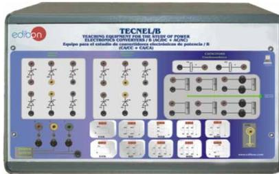
① Unit: TECNEL/B. Basic Teaching Unit for the Study of Power Electronics (no IGBTs), including Control Interface. (Converters: AC/DC+AC/AC).
