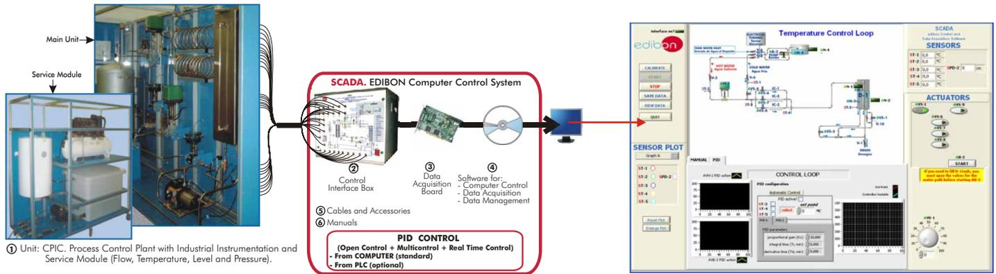
① Unit: CPIC. Process Control Plant with Industrial Instrumentation and Service Module (Flow, Temperature, Level and Pressure).
