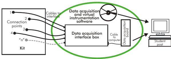
EDAS/VIS is the perfect link between the modules and the PC. With the EDAS/VIS system, information from the modules is sent to the computer. There, it can be analyzed and represented.
