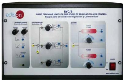
RYC/B allows the user to learn the basics about regulation and control of first and second order systems. This unit enables to carry a set of practices related with basic regulation and control, through which the user will understand how to characterize first and second order systems and how a PID controller works.
