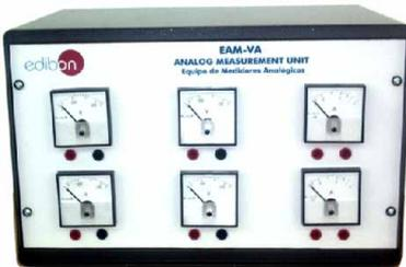
This unit allows to analyze the different voltages and currents involved in a circuit through a simple frontal panel that includes analog measurement instruments.
