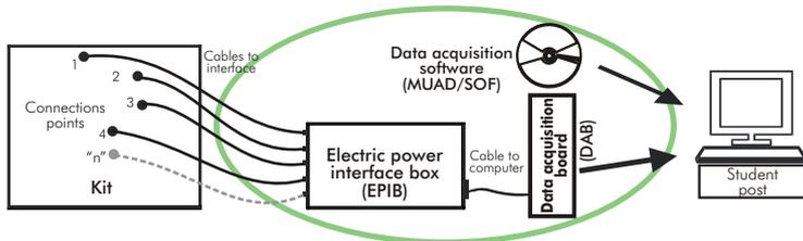
MUAD is the perfect link between the kit/application and the PC. MUAD is a continuous data acquisition system with virtual instrumentation, that measures, analyzes and represents the parameters involved in the process.
