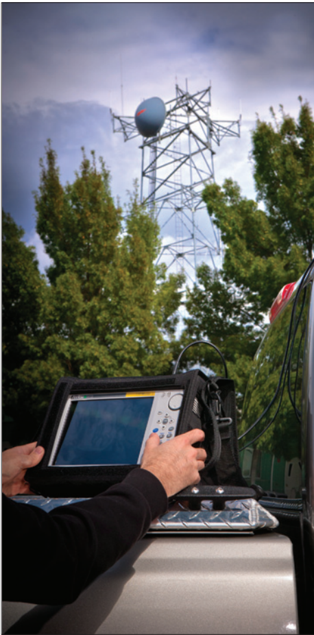
LMR Master testing from a service vehicle
