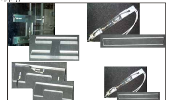
EFO-K4. Kit of Test Specimens with Strain Gauges (advanced kit)
