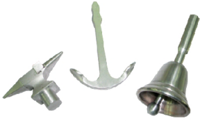
Detail of the finished, fettled castings
