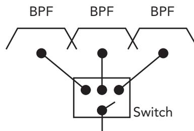
The filter bank technique uses a set of Band Pass Filters (BPF), and these each have typically a bandwidth of 400 MHz. A switch is then used to select a matrix of different BPF to give the required high band selectivity. These filters are implemented using printed circuit techniques, to give low cost, low power consumption, and high stability. The stability comes from there being no tuneable or variable circuits involved.
