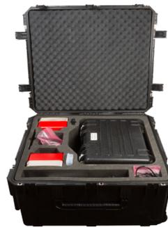
All items required to test radio altimeter systems are included in the ALT-9000 kit.
