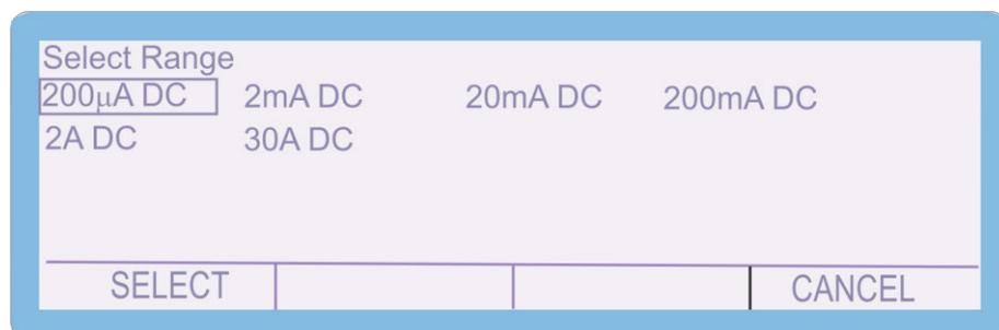
3. The Calibrator will now change to the 200uA DC range. Use the Range Up / Range Down keys to select the Positive Full Scale adjustment point
