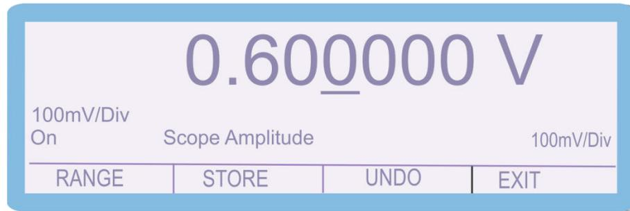
If required, adjust the output as previously described, either typing in the measured value or deviating the output of the calibrator using the cursor and the arrow keys / digital control.
