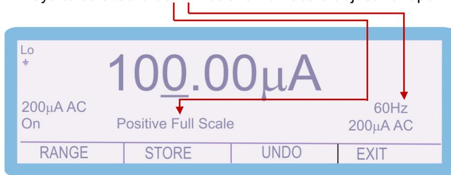
4. Connect the calibrator output voltage terminals to the precision multimeter. Ensure that the multimeter is in AC Current on the appropriate range. Ensure that the correct terminals / current shunt is used for the various current outputs. The 3000A calibrators can output up to 30A AC current, which can blow the fuse / cause damage if the incorrect input is used
