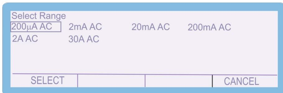
3. The Calibrator will now change to the 200uA AC range. Use the Range Up / Range Down keys to select the 60Hz Positive Full Scale adjustment point
