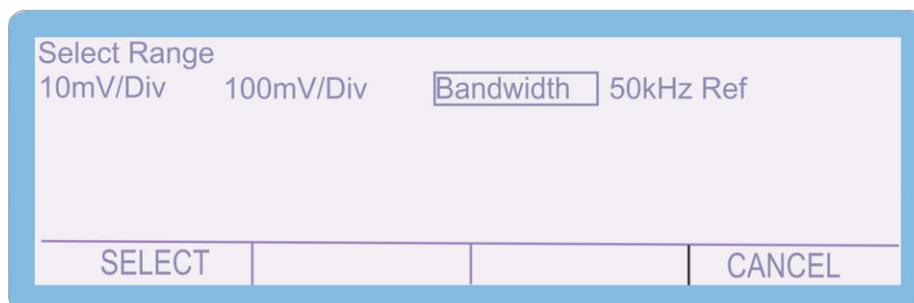
3. The Calibrator will now change to the Scope Bandwidth Function. Use the Range Up / Range Down keys to select the required Scope Bandwidth adjustment point
