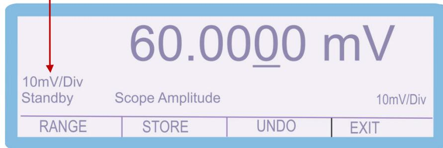
4. Connect the calibrator Oscilloscope output to the precision digital multimeter. Set the 100mV DC voltage range. Normally the Oscilloscope Amplitude output is a levelled square AC Voltage output, however in the calibration mode this is set to a levelled DC waveform. This allows more accurate measurement than low level AC Voltage measurements
