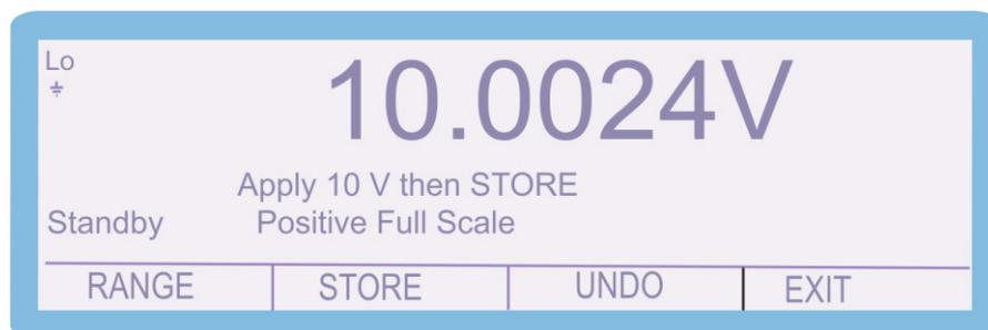
4. Apply an output of 10V from your voltage source to the adapter interface, using Pin 7 as the Ground or Negative connection, and Pin 9 as the Signal or Positive connection.
