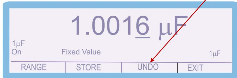
This will remove any changes that have been made to the output of the calibrator.
