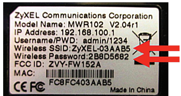
Figure 3. The Pocket Router configuration information.
