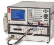
The RCTS-012 Radio Communications Test Set is used to test the AN/ARN-89, AN/ARN-123, AN/ARN-147 and AN/ARN-149 avionics/navigation radios.
