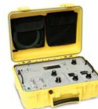
The PSD60-2R is an accurate, highly reliable, portable capacitance test set. Along with an aircraft specific interface, the PSD60-2R will test any AC capacitive fuel, water, LOX, engine oil or other AC capacitance system.
