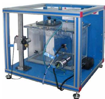
① Unit: QDTGC. Gaseous Mass Transfer and Diffusion Coefficient Unit
