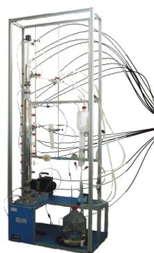
① Unit: UDCC. Continuous Distillation Unit
