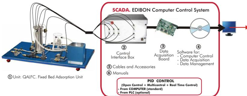
① Unit: QALFC. Fixed Bed Adsorption Unit
