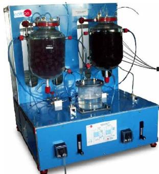
① Unit: PDANC. Anaerobic Digester
