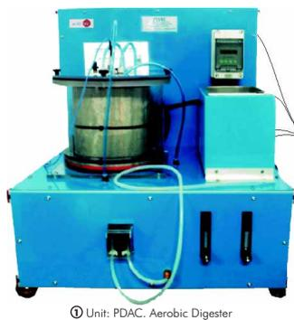
① Unit: PDAC. Aerobic Digester
