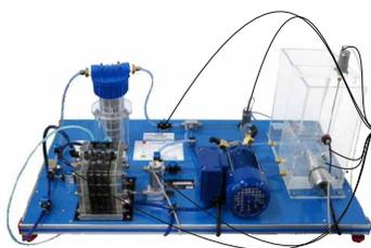
① Unit TFUC. Continuous and Batch Filtration Unit
