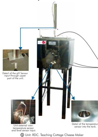
Detail of the pH Sensor input through upper part of the unit.
