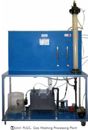
① Unit: PLGC. Gas Washing Processing Plant
