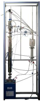
① Unit: UDDC. Batch Distillation Unit
