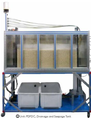
① Unit: PDFDC. Drainage and Seepage Tank
