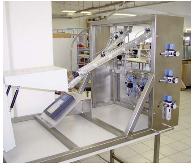
Mechanical life test of the 4921 RF Shield
