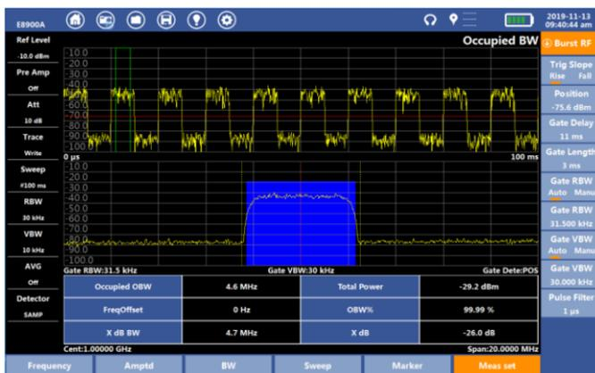
Fig.3-15 Burst RF setting
