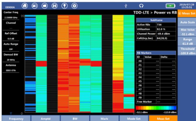
Fig.5-1 RB power test
