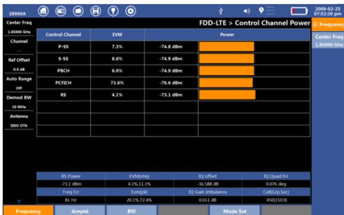
Fig.6-3 Control power measurement
