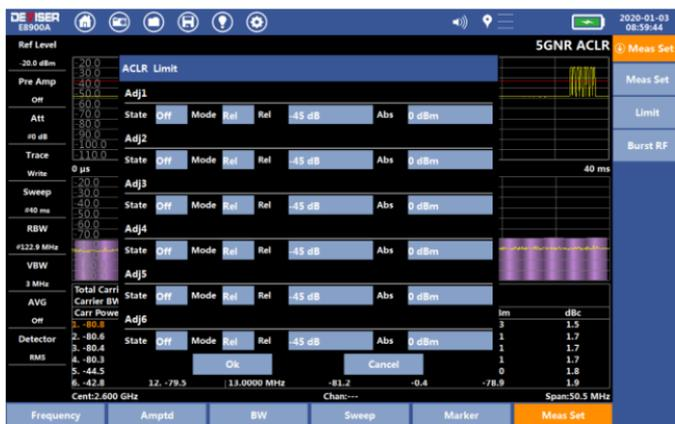
Fig.8-29 5G ACLR Measurement setting
