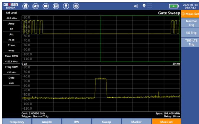
Fig.3-28 Measurement setting
