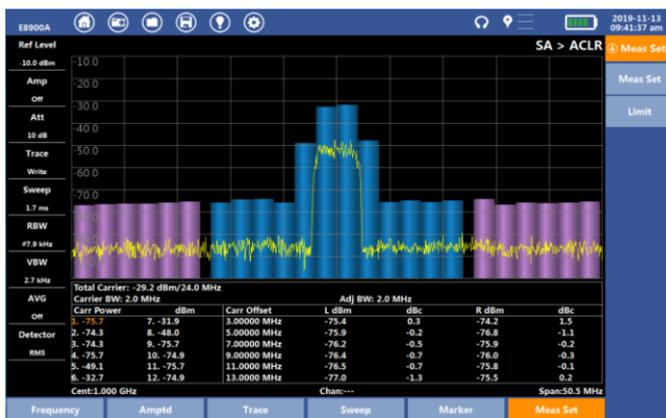
Fig.3-16 ACLR measurement
