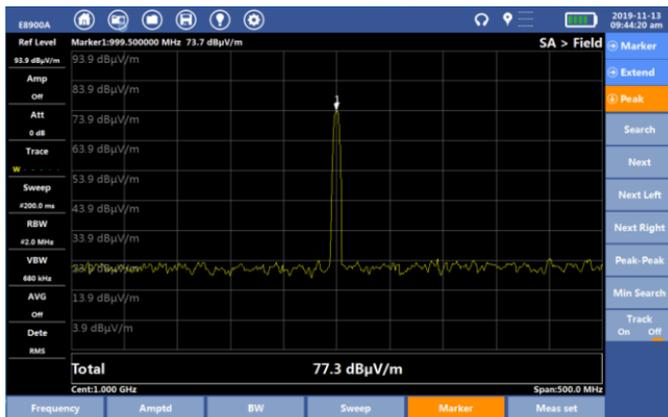
Fig.3-21 Field Strength Test
