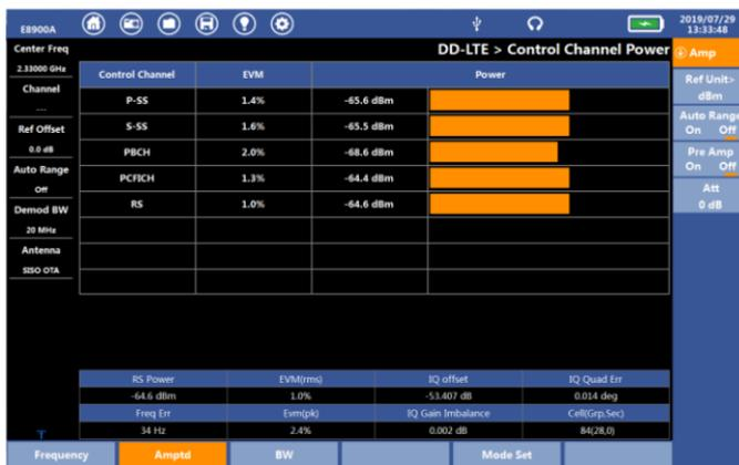
Fig.5-4 Control CH Power
