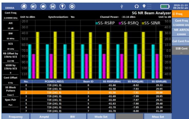
Figure.8-19 5G-NR Beam Analyzer
