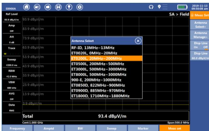
Fig.3-20 Field Strength Antenna List
