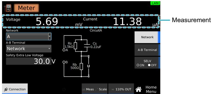
If Measuring across terminals A and B (A-B Terminal) (p.173) is set to VoltMeter and voltage exceeding the value set with SELV setting (p.174) is present across terminals A and B, the DANGER LED lights.
