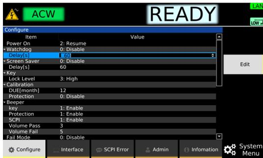
**5 Use the numeric keypad or the rotary knob to enter the duration of time until the product decides that there is no SCPI communication, and then press ENTER.**
