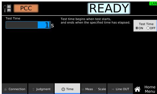
**2** Press Test Time to switch between on and off.
