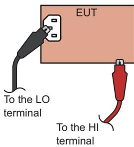
Ex: Between the protective ground terminal and grounded enclosure
