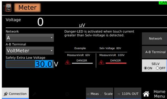
**4 Use the numeric keypad or the rotary knob to enter the voltage limit.**
