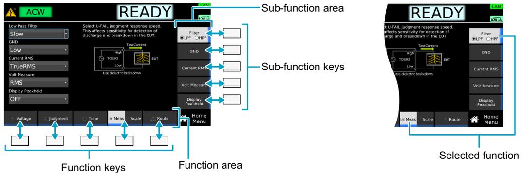
If several functions are displayed for a single key, the function switches each time you press the key.
