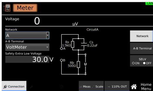
**8 Press A-B Terminal, and then turn the rotary knob to select Network.**
