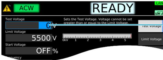
Use the numeric keypad or the rotary knob to change the value.
