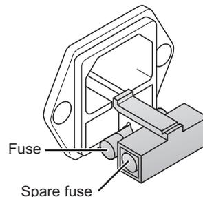
**3** Replace the blown fuse with an appropriate one.
