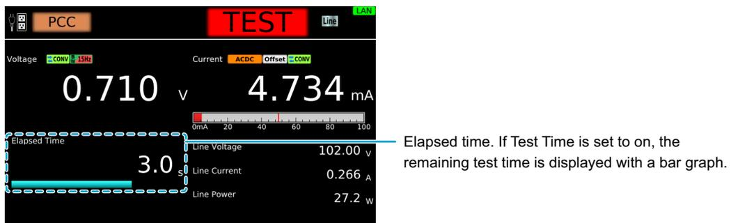
Elapsed time. If Test Time is set to on, the remaining test time is displayed with a bar graph.
