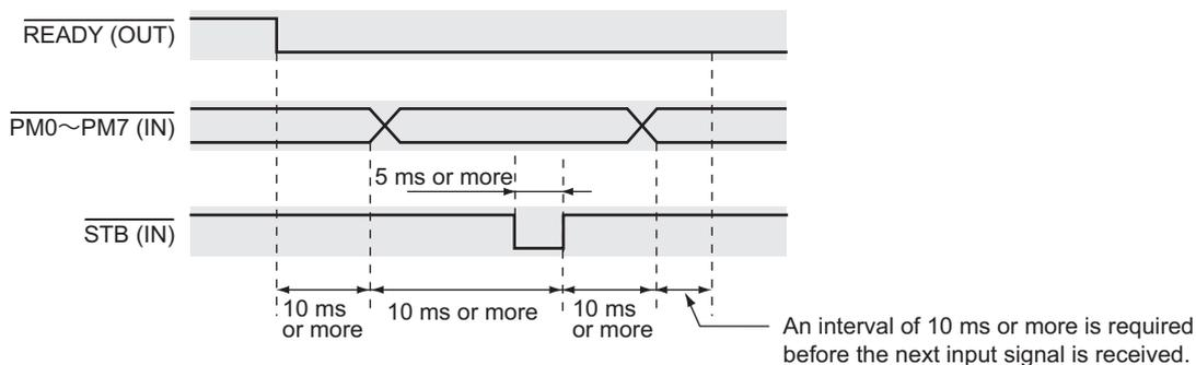
**1** With “READY” shown in the upper right of the display, apply high-level or low-level signals to PM0 (pin 3) to PM7 (pin 10) of the SIGNAL I/O connector.
