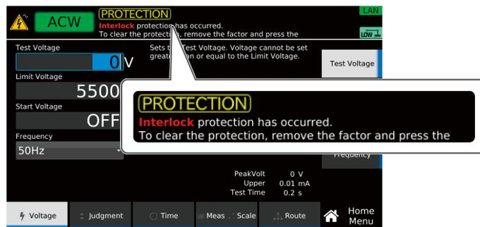
This completes the checking of the interlock operation.
