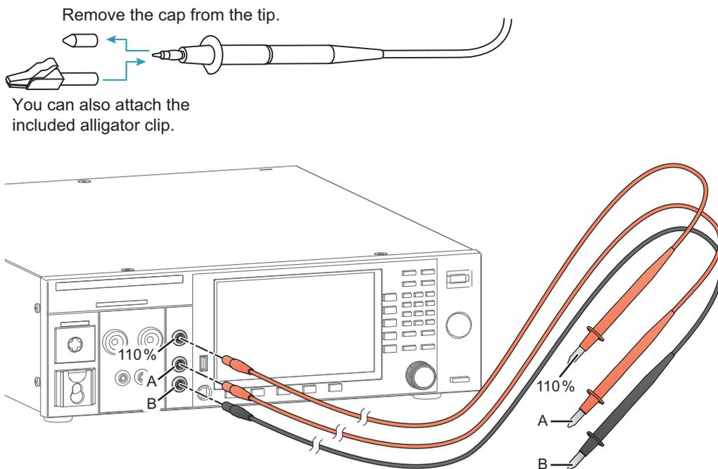
The locations on the EUT that test leads are connected to vary depending on the probe and condition settings of the test conditions and the appliance class of the EUT. For details on touch current testing, see “Connecting the test leads to the EUT” (p.120). For details on patient leakage current testing, see “Connecting the test leads to the EUT” (p.162).
