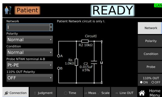
Set the required conditions by referring to the description of test conditions (p.147).
